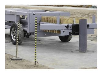
Our comprehensive testing program specifically addresses the growing demand for protective devices under dynamic impact conditions, ensuring thorough compliance with the ASTM F3016 "Standard Test Method for Surrogate Testing of Vehicle Impact Protective Devices at Low Speeds."
